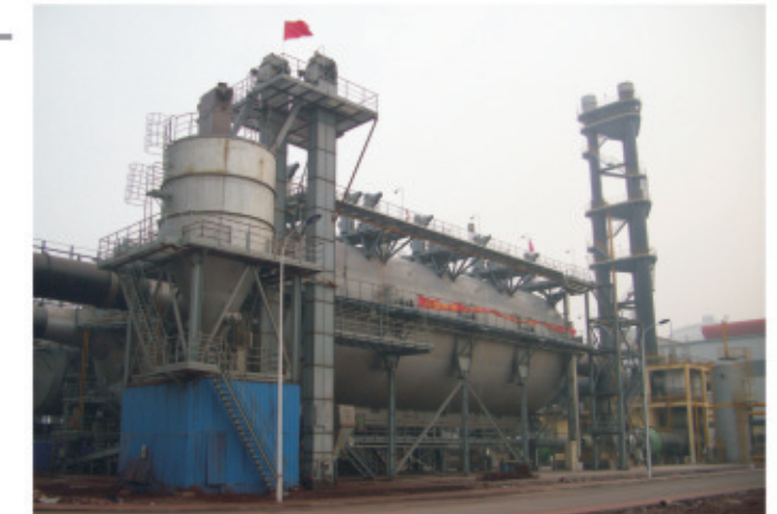
BFG dry bag filter for Baosteel No.1 BF revamp – China's first BFG dry bag filter application to mega blast furnace
