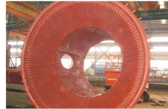
Converter Waste-heat Boiler (Hood)
