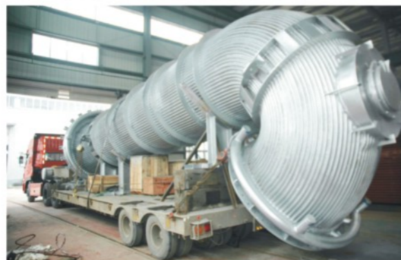
Tail Section of 50t Converter Waste-heat Boiler
