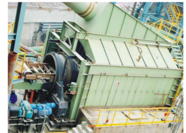
CISDI Slag Granulating Drum Equipment
