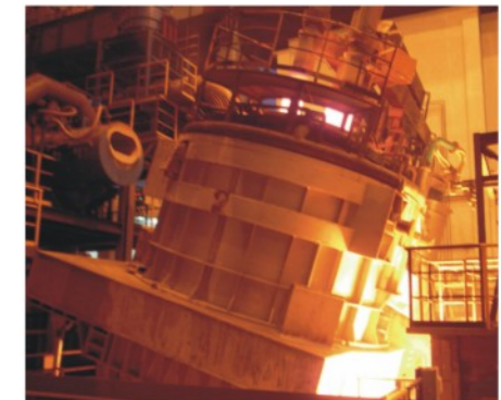
Electric Furnace Using Recycled BF Slag
